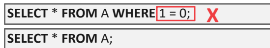
Figure 4: Unnecessary Predicates – The predicate in the first query will always be false and can be disregarded. The next predicate will always return true and can also be bypassed.
